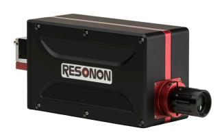
The Pika UV (formerly Pika NUV2) is a line-scan hyperspectral camera that covers the near ultraviolet and visible spectral range (330 – 800 nm). The Pika UV is the only ultraviolet + visible hyperspectral camera commercially available. It can be used with Resonon's Reflectance benchtop system, outdoor, and airborne systems, standalone with our software development kit, and integrated into machine vision systems.
