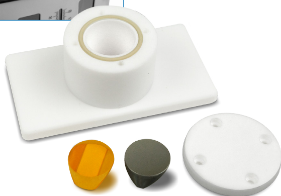
VeeMAX III spectroelectrochemical cell – maximum flexibility with its interchangeable and removable crystals.
